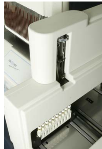
Figure 2 – Close up of the Rack loader
