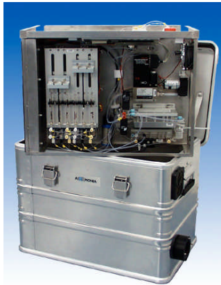
The AiRRmonia is installed in an Aluminium, ruggedized, weatherproof box.
